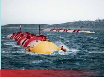
Figure 6: "P2" electricity generator
