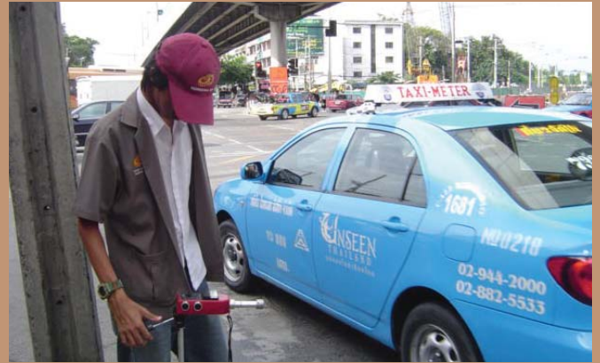
Figure 3 : Method of Application of Sound Level Meter
